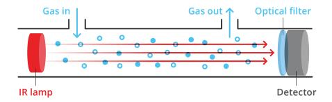
Aranet4 uses the nondispersive infrared (NDIR) sensor to measure the concentration of  $CO_2$ . The  $CO_2$  gas in the chamber absorbs infrared light and this absorption is measured by the sensor. The less light passes through – the higher the  $CO_2$  concentration. The  $CO_2$  gas absorbs only a specific wavelength of the light therefore an optical filter is used.
